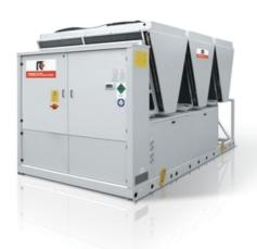
Outdoor unit for the production of chilled water with hermetic rotary Scroll compressors, ozone-friendly refrigerant R410A, axial-flow fans, shell and tubes exchanger and electronic expansion valve. The range is composed by units equipped with four, six and eight compressors in multi-circuit configuration.
